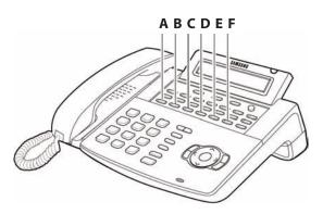
pulse to tone conversion. If your system uses rotary (or pulse) dialing C.O. lines, pressing **D** while entering a speed dial number causes all subsequent digits to be sent as DTMF tones.
